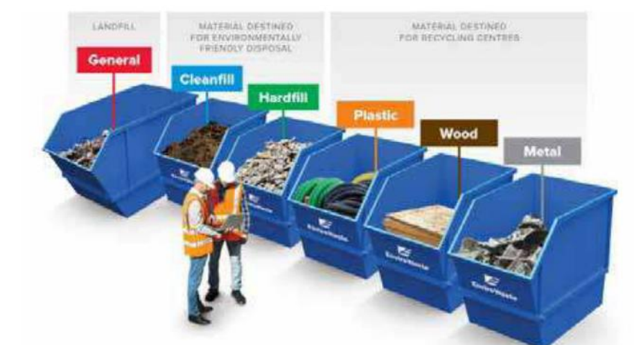
Waste separation as part of SWMP
