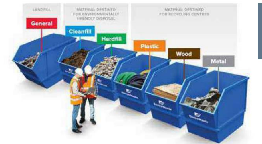
Waste separation as part of SWMP
