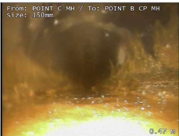
Water level 25% height/diameter, Start
