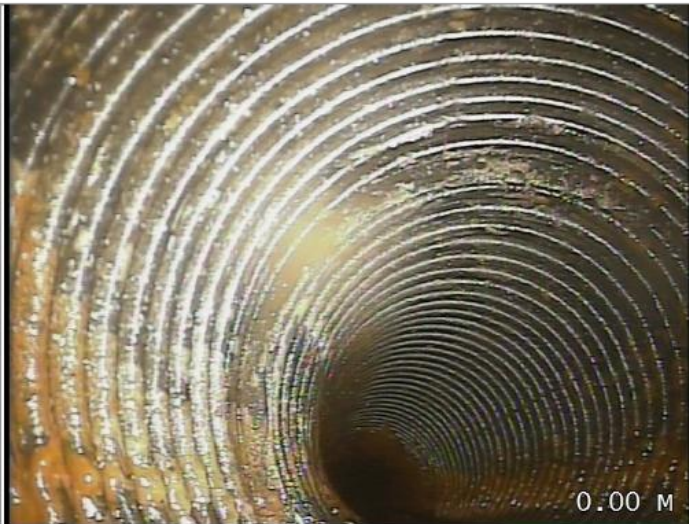
Water level 5% height/diameter
