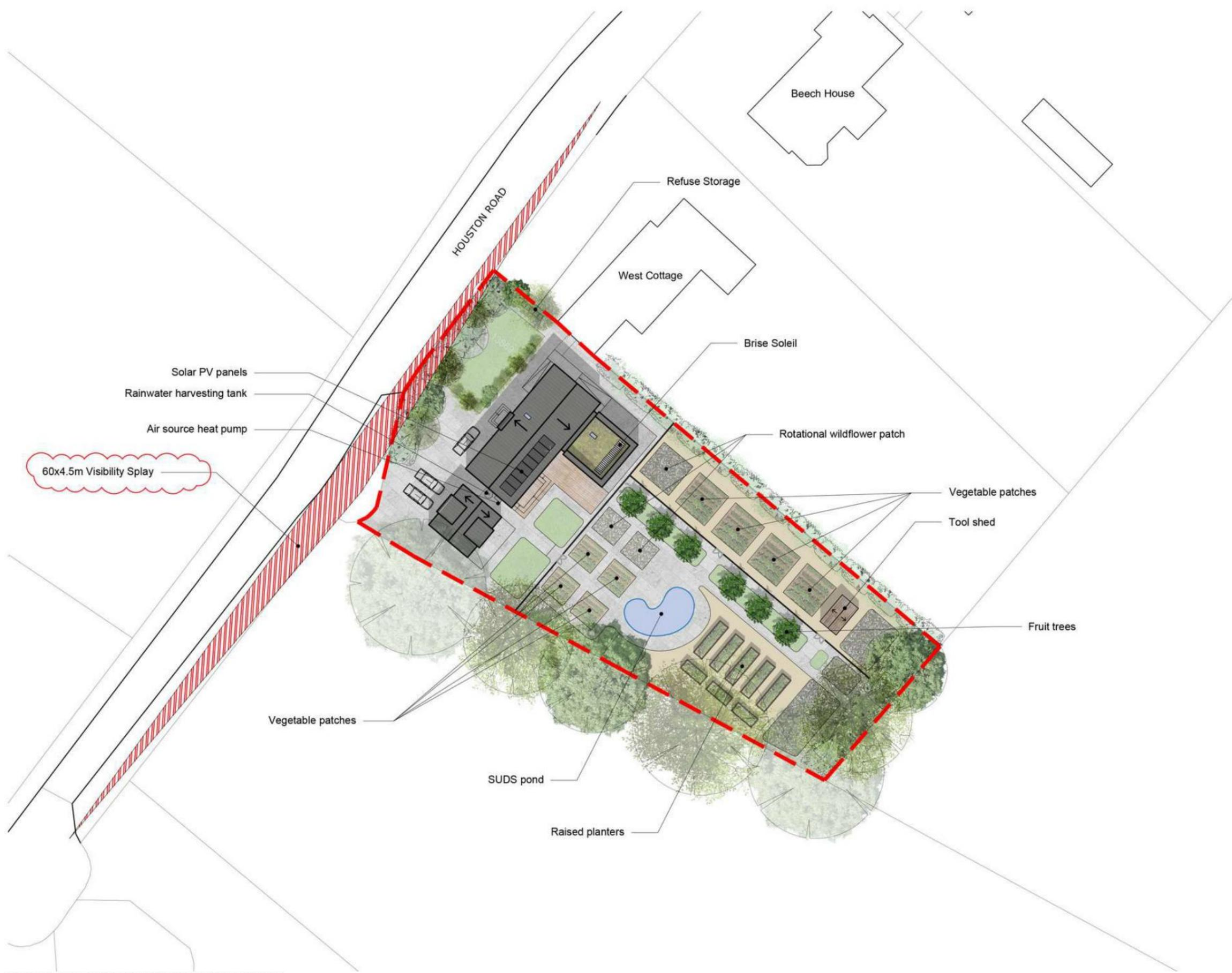
**PROPOSED SITE PLAN SHOWING ROOF**
