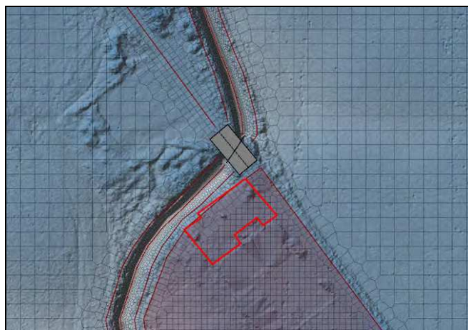
Figure F – Extract of 2D Geometry with Computational Mesh
