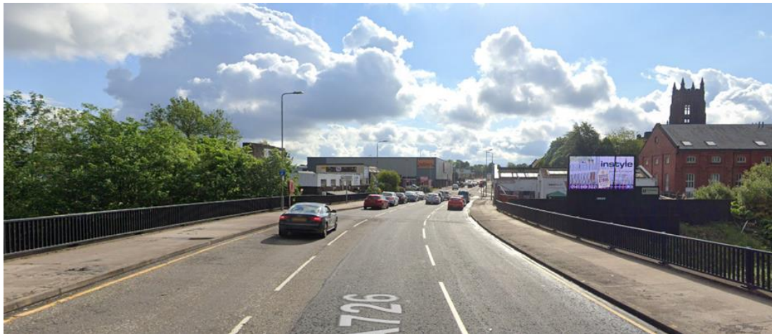
Example 1; An acceptable location where the screen is off to the side and does not interfere with the visibility of the signal heads.
